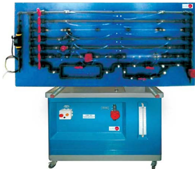
① Unit: AFTC. Fluid Friction in Pipes, with Hydraulics Bench (FME00)
