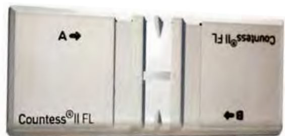
Figure 2. Reusable slide for the Countess II FL Automated Cell Counter helps reduce consumable costs.
