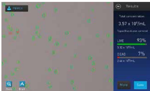
Figure 1. PBMCs counted using the Countess II Automated Cell Counter. Counting and viability measurement can be done using standard trypan blue staining. The results screen displays total concentration and percentage of live and dead cells.
