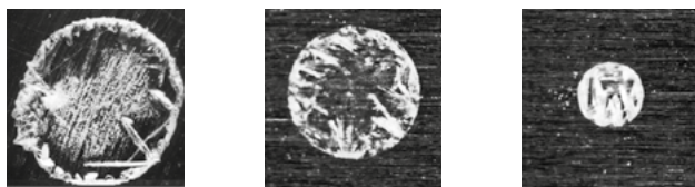
Depending on the sample type, a larger or smaller diameter AnchorChip target may be selected. The examples above demonstrate crystallization of DHB to a standard stainless steel, 800 mm and 400 mm AnchorChip targets (left to right).
