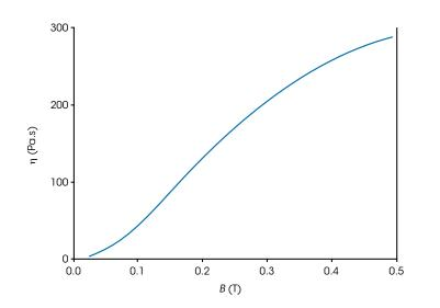
• Viscosity shows a significant response to step changes in magnetic field
