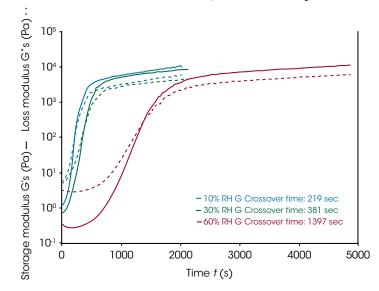
Tensile modulus of Fuel Cell Membrane - Humidity Effects
