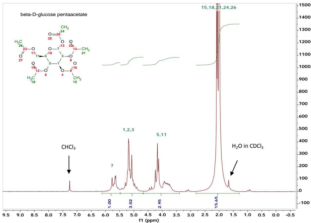
**Fig.7: Assigned and integrated 60MHz <sup>1</sup>H-NMR spectrum of β-D-glucose pentaacetate.**
