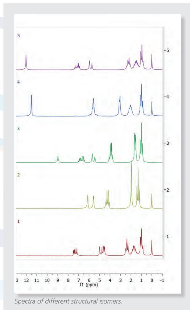
The spectral data obtained on **Pulsar** shows clear separation of the multiplets commonly observed in NMR spectra. The example above shows the typical multiplets generated by hydrogen atoms in an ethyl ( $\text{CH}_3\text{CH}_2-$ ) group in the molecule.
