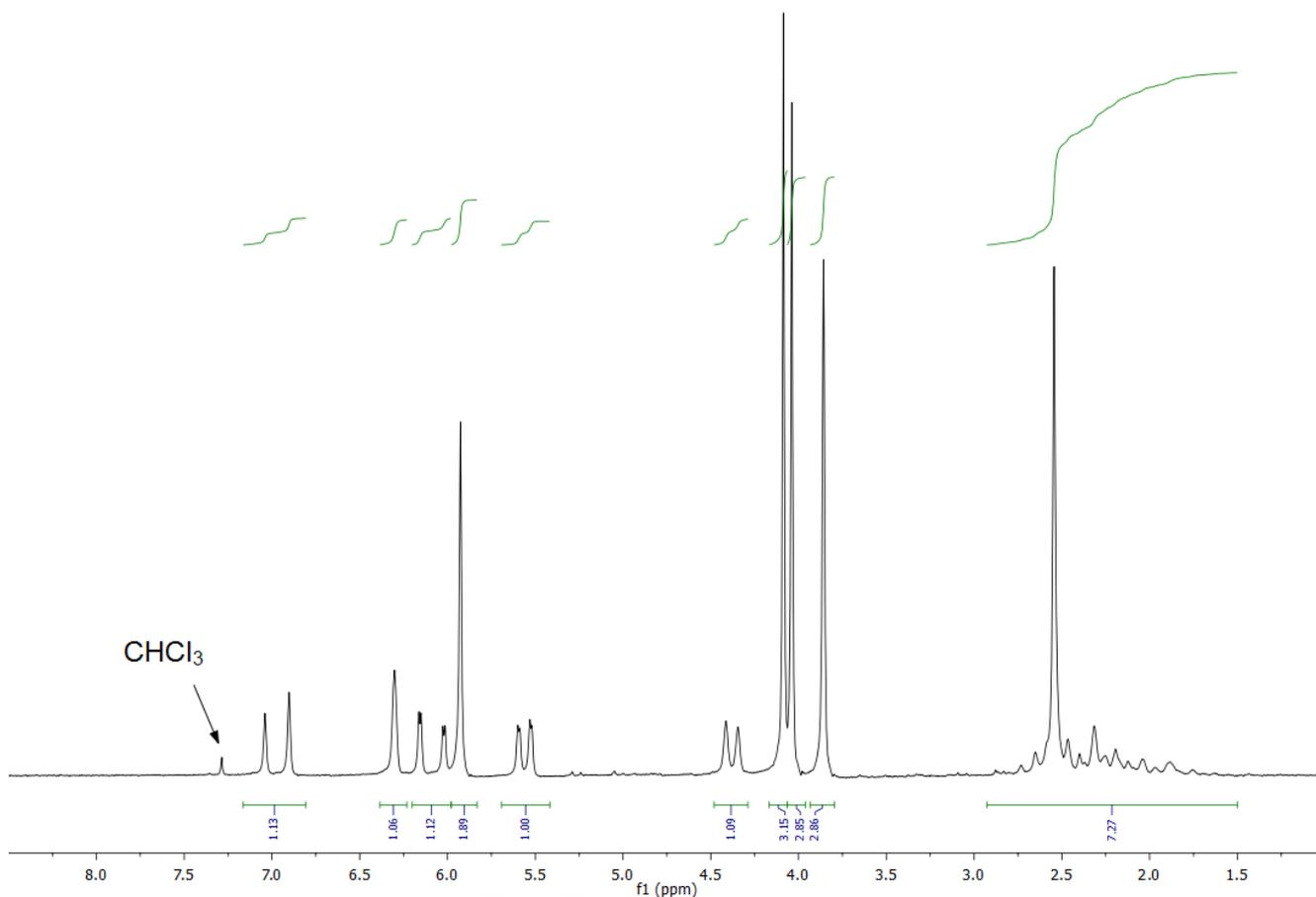
Figure 5:  $^1\text{H}$  spectrum of 259 mM noscopine in  $\text{CDCl}_3$  shown in Figure 4 acquired with 64 scans, after the application of reference deconvolution with a target linewidth of 0.50 Hz, using TMS as a reference. Integrals of the sample peaks are shown; the methyl peak at 2.08 ppm was normalized to an area of 3.00. The processing parameters were identical to those used in Figure 2, except no exponential function was applied.
