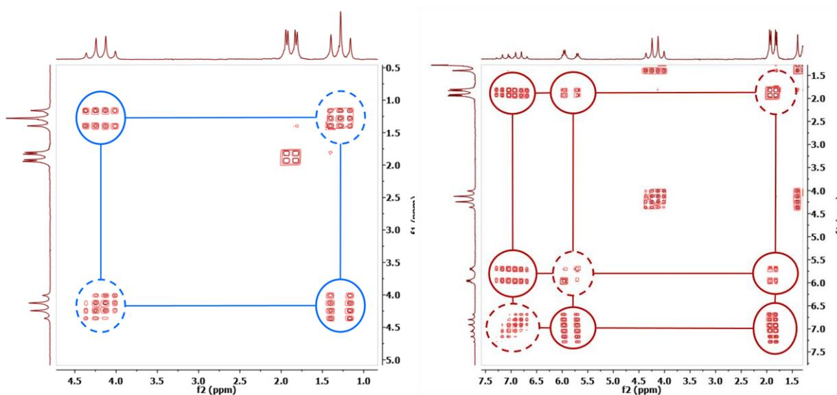
Figure 4: Expanded regions of the COSY spectrum showing the ethyl region of the spectrum (left) and the crotonate region (right). The diagonal peaks are highlighted as dashed circles and the cross peaks are highlighted with full circles.
