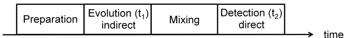
Figure 1: schematic representation of a 2D NMR experiment
