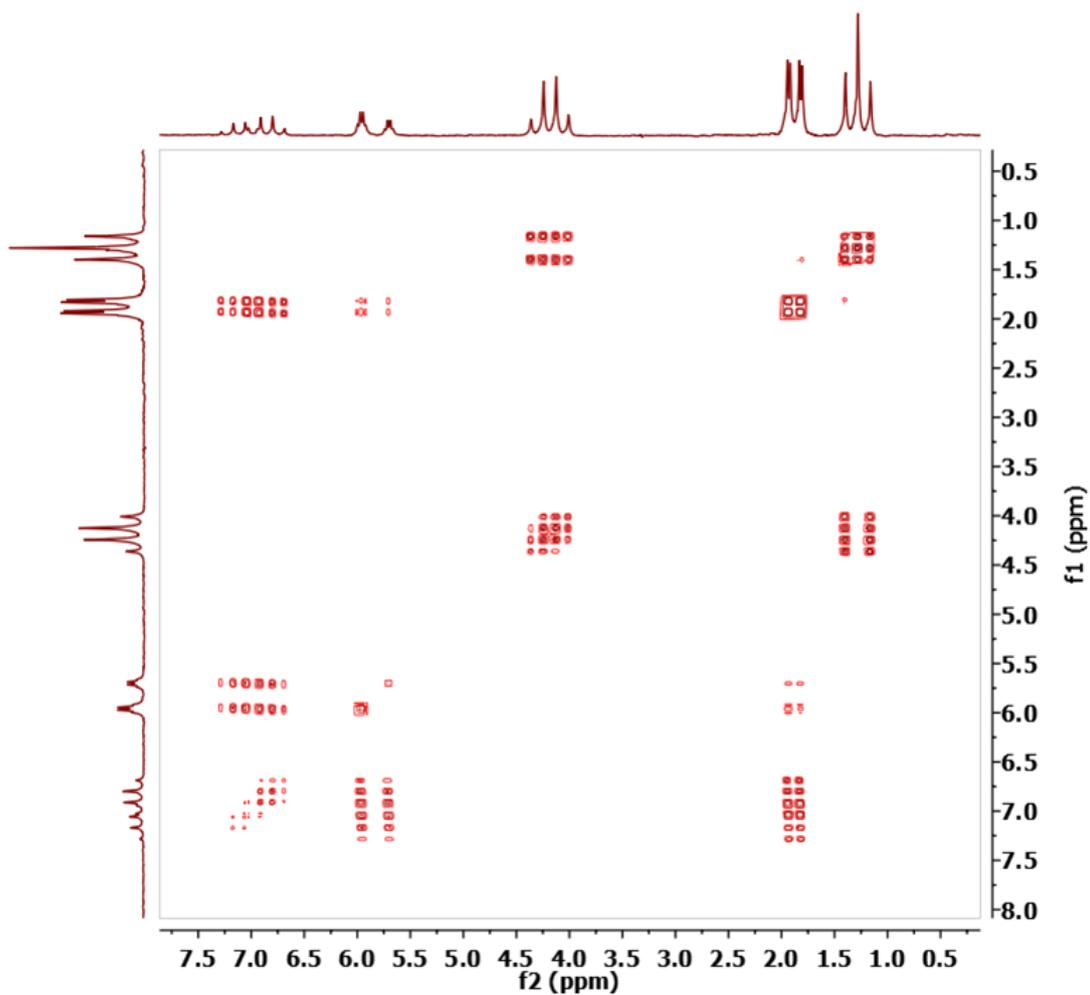
Figure 3: Full COSY spectrum for ethyl crotonate. All peaks in the 1D spectrum show a diagonal peak in the COSY and the cross peaks (off diagonal peaks) show coupling between the particular chemical shifts,
