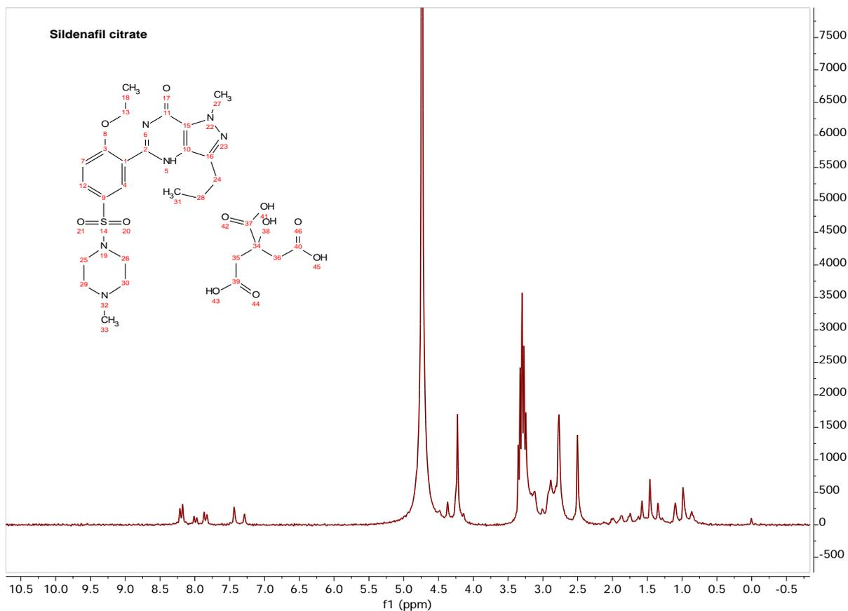
**Fig.6: 60MHz  $^1\text{H}$ -NMR spectrum of sildenafil citrate in methanol- $\text{d}_4$  (around 9 mM).**
