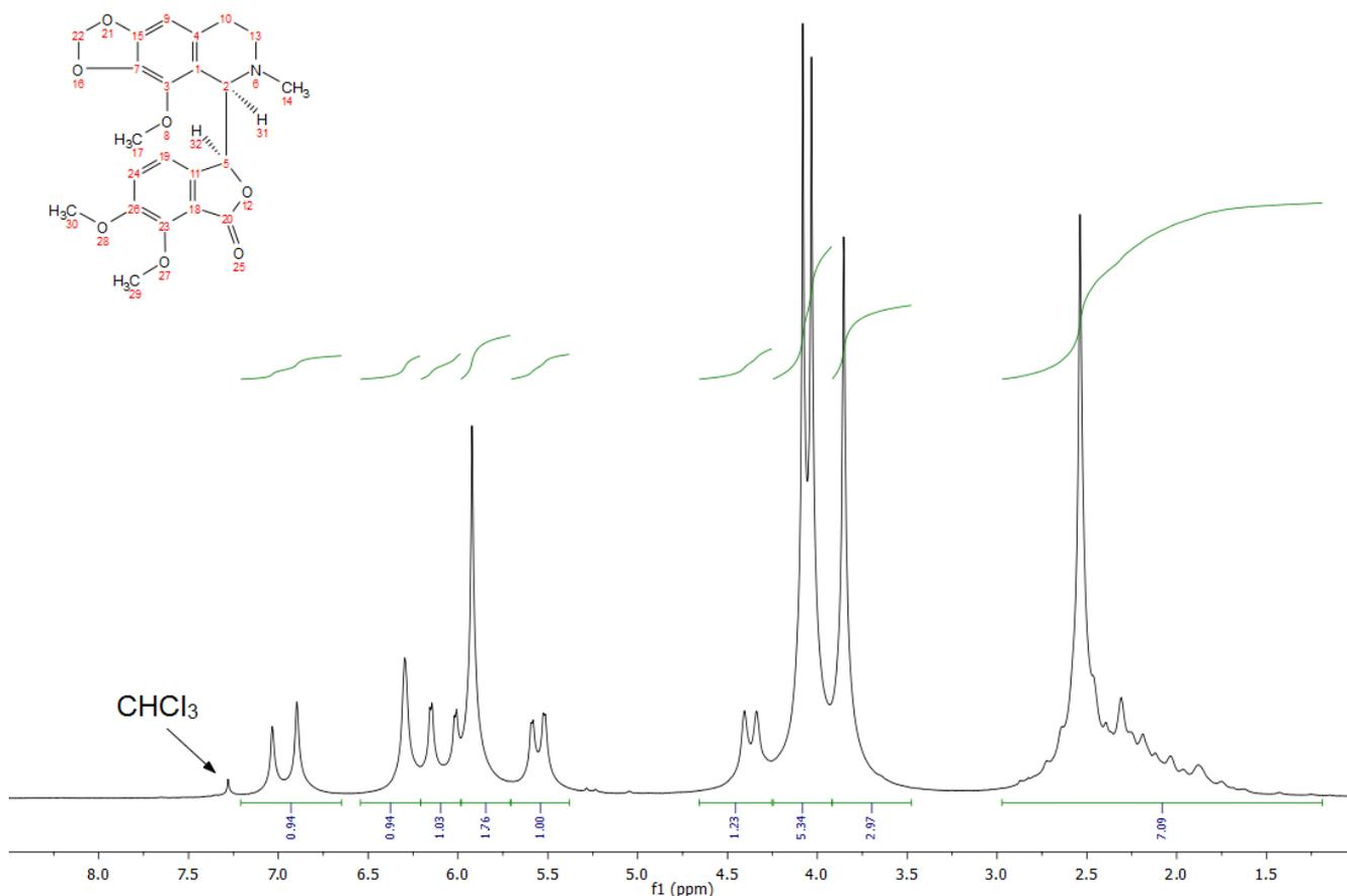
Figure 4:  $^1\text{H}$  spectrum of 259 mM noscapine in  $\text{CDCl}_3$  (99.8% D, Sigma-Aldrich). Integrals of the sample peaks are shown; the doublet at approximately 5.5 ppm was normalized to an area of 1.00. Chemical shifts were referenced to TMS at 0 ppm. 128 scans were acquired. The spectrum was zero-filled to 256k points; 3<sup>rd</sup> order polynomial baseline correction and a 0.1 Hz exponential function were applied.
