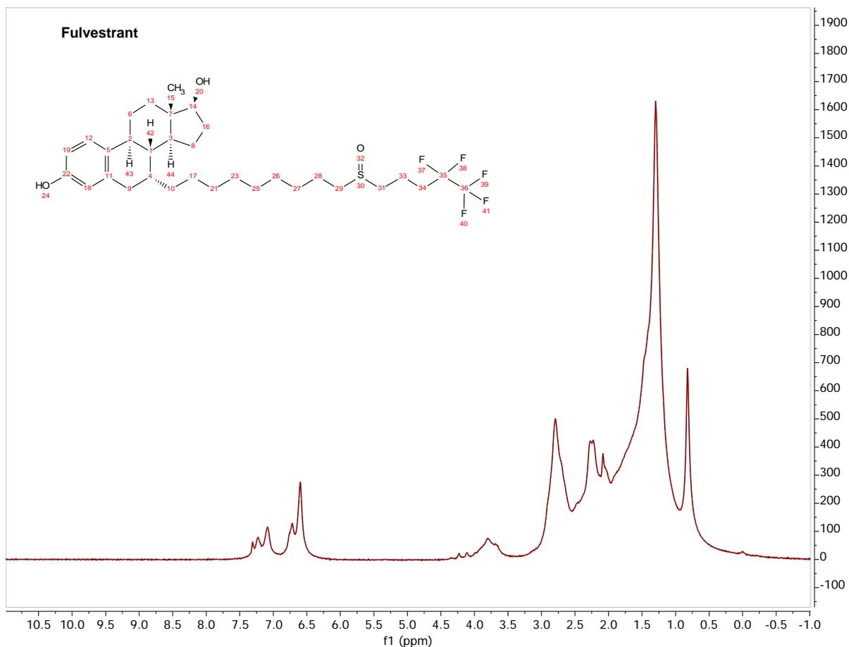
**Fig.4: 60MHz  $^1\text{H-NMR}$  spectrum of fulvestrant in  $\text{CDCl}_3$ .**
