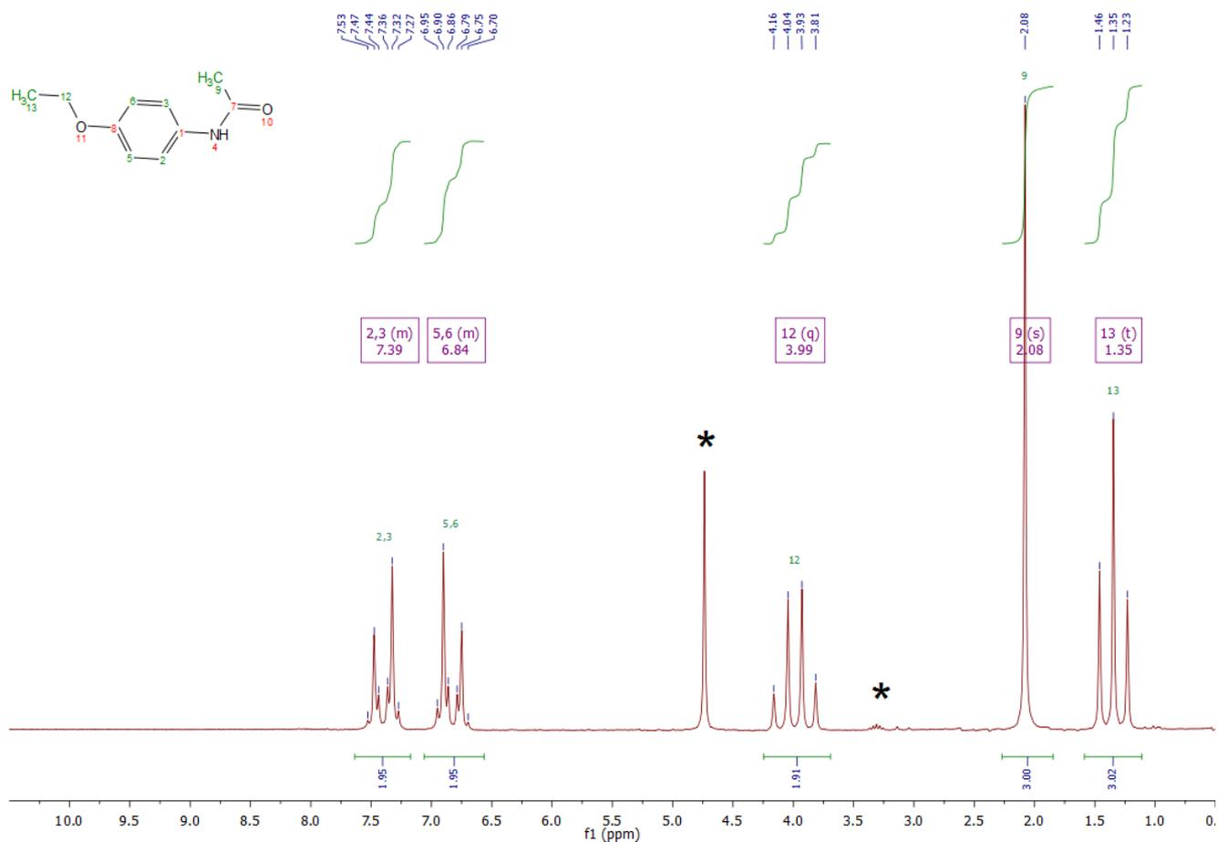
Figure 3:  $^1\text{H}$  spectrum of 290 mM phenacetin in methanol- $d_4$  as in Figure 2, after the application of reference deconvolution with a target linewidth of 0.50 Hz. Integrals of the sample peaks are shown; the methyl peak at 2.08 ppm was normalized to an area of 3.00. Identical processing parameters were used as in Figure 2, except no exponential function was applied. Asterisks indicate residual solvent peaks.
