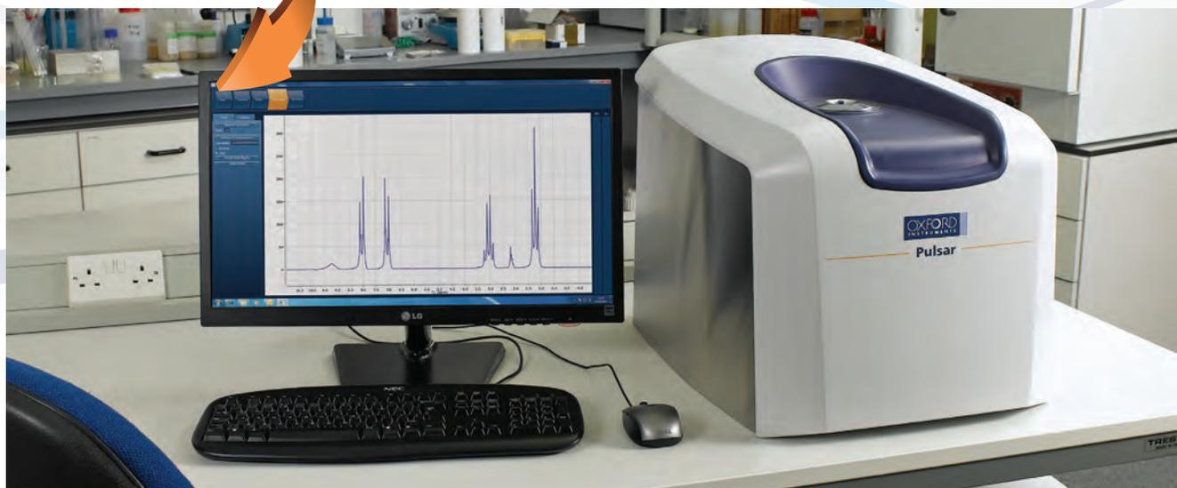
Once the data collection is complete, the spectrum is available for reporting or further data manipulation. **Pulsar** is packaged with a perpetual license for the powerful Mnova software from Mestrelab. This software has a full suite of routines for processing and analysing NMR data, and has a range of spectral display options including 2D and 3D stacking. This is particularly useful for reaction monitoring experiments.
