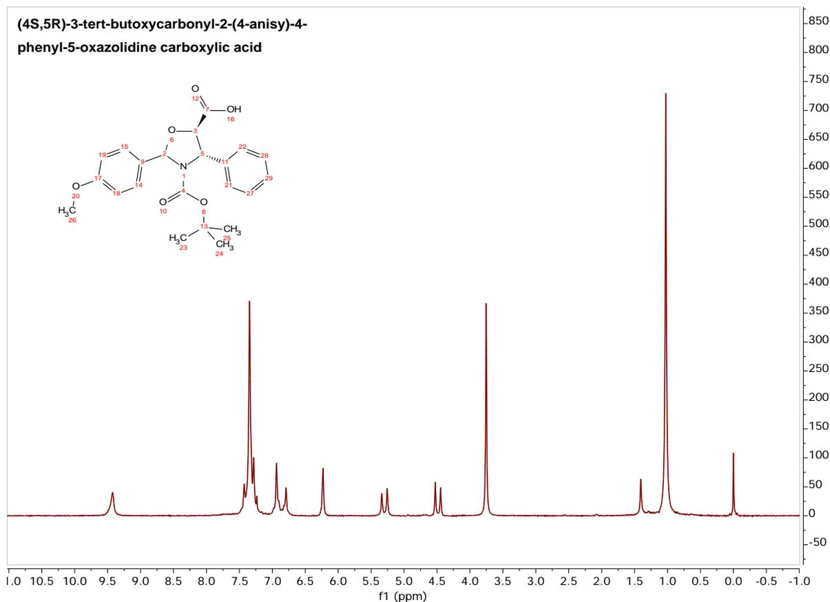
**Fig.5: 60MHz <sup>1</sup>H-NMR spectrum of (4S, 5R)-3-tert-butoxycarbonyl-2-(4-anisyl)-4-phenyl-5-oxazolidine carboxylic acid in CDCl<sub>3</sub>.**
