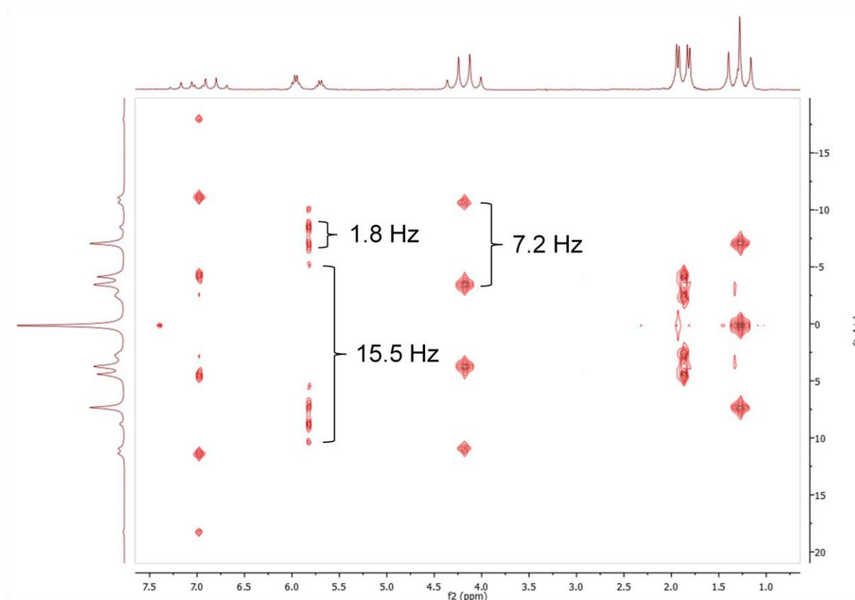
**Figure 5:** Full J-resolved spectrum of ethyl crotonate. The horizontal axis shows the chemical shift information and the vertical axis shows the J-coupling. Some examples of couplings are highlighted
