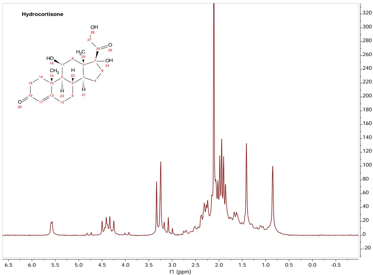
**Fig.1: 60MHz  $^1\text{H}$ -NMR spectrum of hydrocortisone in ACN.**
