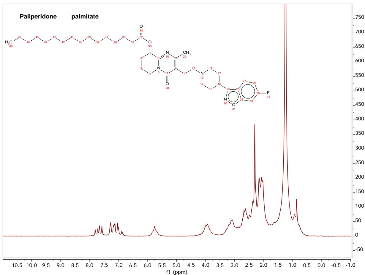
**Fig.2: 60MHz <sup>1</sup>H-NMR spectrum of paliperidone palmitate in CDCl<sub>3</sub>.**
